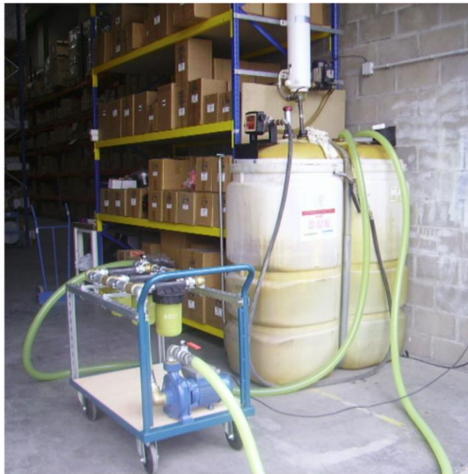
Model DEP280 Cleaning a 1000 Litre Tank (280 LPM Flow)
